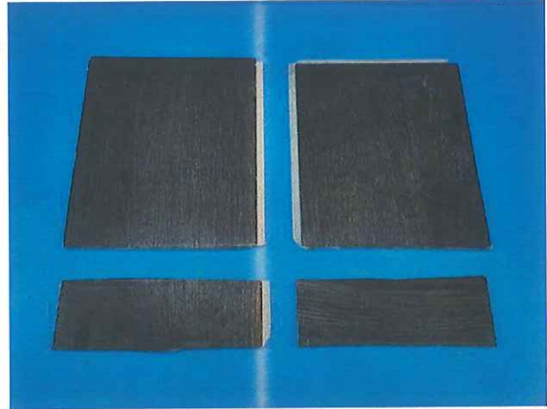
After the hot air aging test
