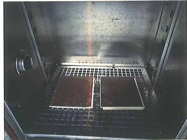
Dimensional stability test after hot air aging
