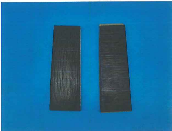
After water absorption thickness expansion rate test
